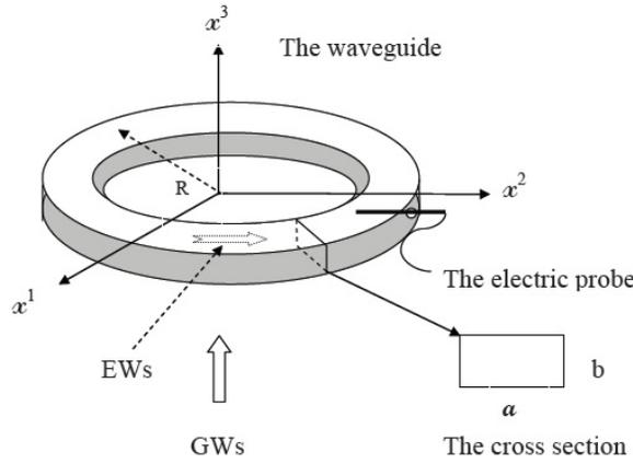
**Fig. 2** A sketch of the annular waveguide. The cross section of the waveguide is a rectangle with side  $a$  and  $b$  which are much smaller than the radius  $R$ . EWs travel inside the waveguide and GWs propagate along the  $x^3$ -axis.
